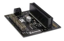
Take your robotics project to the next level with the (i2C) Kitronik 16 Servo Driver Board for the BBC micro:bit. Capable of controlling 16 servos which are powered directly from the board's power supply. **More Info**
