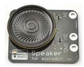
The MonkMakes Speaker for micro:bit is a neat little amplified speaker that connects to your micro:bit using alligator clips. Despite its small size, this speaker is pretty loud.
