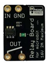
The MonkMakes Relay for the BBC micro:bit is a solid-state (no moving parts) relay that allows an output of a micro:bit to turn things on and off.
