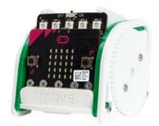
The :Move mini is a 2 wheeled robot that is suitable forautonomous operation, remote control projects via a Bluetooth application or being controlled using a second BBC micro:bit as a controller via the microbits radio functionality.
