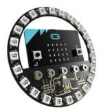
The Halo has 24 ZIP LEDs, which are individually addressable full colour LEDs. This means that each LED can display a huge spectrum of colours, allowing amazing colourful effects to be achieved.
