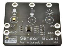
The Monk Makes Sensor Board for micro:bit allows you to sense sound levels, temperature and light levels.
