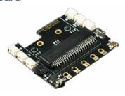
Comes with 6 fool-proof 3-Pin sockets, compatible with hundreds of DFRobot's Boson modularized electronic blocks, covering popular digital and analog sensors and actuators, supporting sound, light and motion interaction. **More Info**
