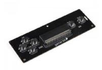
The SparkFun gamer:bit is a fun-filled "carrier" board for the micro:bit that, when combined with the micro:bit, provides you with a fully functional game system.
