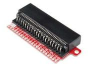
This breakout boards edge connector allows intermediate and advanced users to connect the micro:bit to breadboards and other sensors, motors, LEDs and more!
