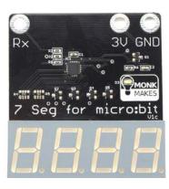
The 7-segment for micro:bit is a four digit 7-segment display for the micro:bit. You can use it to display numbers, letters and other characters, albeit with the limits imposed by the 7 segments of each digit. Powered directly from micro:bit pins it can be used to send messages to the display using the micro:bit's serial blocks.
