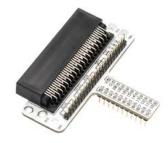
Elecfreaks Breadboard Adapter is a breadboard pinboard created for the BBC micro:bit. It can be directly plugged into a breadboard.
