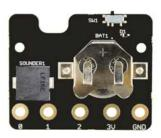
The Mi:power board for the BBC micro:bit brings real portability to your wearable projects. The stylish, lightweight PCB is designed to fit snugly against the BBC micro:bit and features a built in buzzer and 3V coin cell holder.
