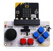
Elecfreaks Joystick: bit is a game joystick for the BBC micro:bit. On the board, it has an integrated joystick and 6 undefined keys.
