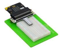
Includes a breadboard, breakout board and a USB cable. Perfect for quick prototyping.
